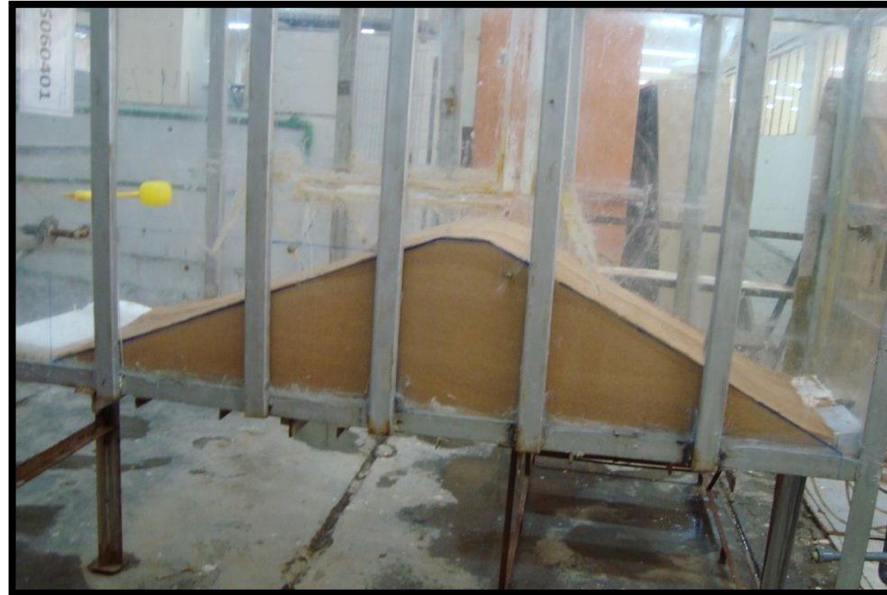
The homogeneous earth dam
